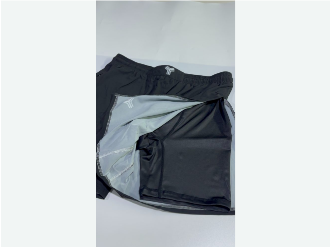
Actual high-split sample: separate outer shell and inner layer.
